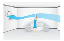
The airflow is directed downwards in heating mode.
